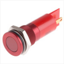
RS PRO Red Indicator, 220 V ac, 14mm Mounting Hole Size, Faston, Solder Lug Termination, IP67, Индикатор Stock number: 1116558
