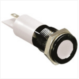
RS PRO White Indicator, 12 V dc, 14mm Mounting Hole Size, Solder Tab Termination, IP67, Индикатор Stock number: 7038888
