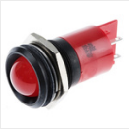
RS PRO Red Indicator, 24 → 36 V dc, 22mm Mounting Hole Size, Tab Termination, Индикатор Stock number: 0212216
