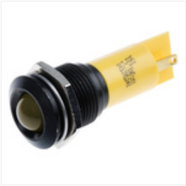
RS PRO Yellow Indicator, 24 V ac/dc, 16mm Mounting Hole Size, Solder Tab Termination, Индикатор Stock number: 0207595
