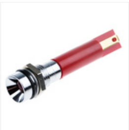
RS PRO Red Indicator, 12 V, 8mm Mounting Hole Size, Solder Tab Termination, IP67, Индикатор Stock number: 0205628
