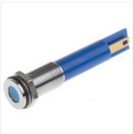
RS PRO Blue Indicator, 110 V ac, 8mm Mounting Hole Size, Faston, Solder Lug Termination, IP67, Индикатор Stock number: 9138738
