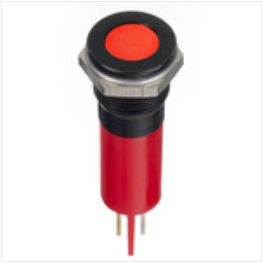
RS PRO Red Indicator, 24 V dc, 12mm Mounting Hole Size, Faston, Solder Lug Termination, IP67, Индикатор Stock number: 1246399
