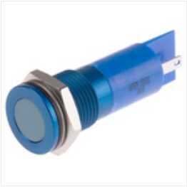
RS PRO Blue Indicator, 12 V dc, 14mm Mounting Hole Size, Faston, Solder Lug Termination, IP67, Индикатор Stock number: 1116565
