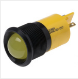
RS PRO Yellow Indicator, 24 V ac/dc, 22mm Mounting Hole Size, Solder Tab Termination, Индикатор Stock number: 0209800
