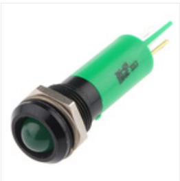
RS PRO Green Indicator, 230 V ac, 12mm Mounting Hole Size, Tab Termination, IP67, Индикатор Stock number: 0206429
