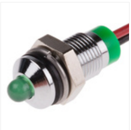
RS PRO Green Indicator, 2 V dc, 6mm Mounting Hole Size, Lead Wires Termination, IP67, Индикатор Stock number: 7227675
