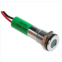
RS PRO Green Indicator, 24 V dc, 8mm Mounting Hole Size, Lead Wires Termination, IP67, Индикатор Stock number: 7001928
