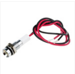
RS PRO White Indicator, 24 V dc, 6mm Mounting Hole Size, Lead Wires Termination, IP67, Индикатор Stock number: 7227772
