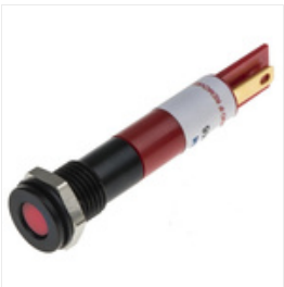
RS PRO Red Indicator, 12 V dc, 6mm Mounting Hole Size, Solder Tab Termination, IP67, Индикатор Stock number: 7001612
