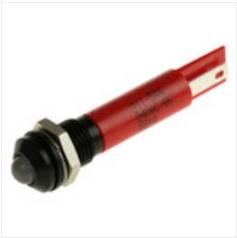
RS PRO Red Indicator, 24 V ac/dc, 8mm Mounting Hole Size, Solder Tab Termination, IP67, Индикатор Stock number: 0211544
