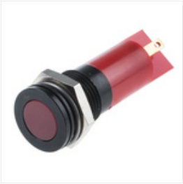
RS PRO Red Indicator, 12 V dc, 14mm Mounting Hole Size, Solder Tab Termination, IP67, Индикатор Stock number: 7038863
