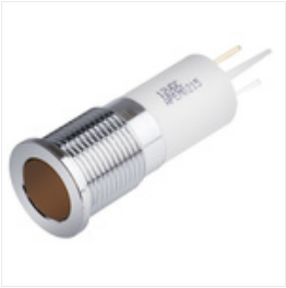
RS PRO Orange Indicator, 10.8 → 13.2 V dc, 14mm Mounting Hole Size, Solder Lug Termination, IP67, Индикатор Stock number: 8432519
