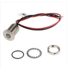
RS PRO White EMC Panel LED, 10.8 → 13.2 V dc, 10mm Mounting Hole Size, Lead Wires Termination, IP67, Индикатор Stock number: 1393379
