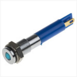
RS PRO Blue Indicator, 12 V dc, 6mm Mounting Hole Size, Solder Tab Termination, IP67, Индикатор Stock number: 7001577
