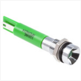
RS PRO Green Indicator, 110 V ac, 8mm Mounting Hole Size, Solder Lug Termination, IP67, Индикатор Stock number: 8462746
