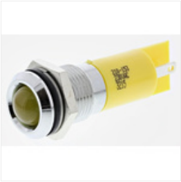
RS PRO Yellow Indicator, 230 V ac, 14mm Mounting Hole Size, Tab Termination, IP67, Индикатор Stock number: 0210153
