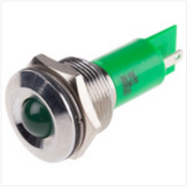
RS PRO Green Indicator, 24 V ac/dc, 19mm Mounting Hole Size, Solder Tab Termination, IP67, Индикатор Stock number: 0206918
