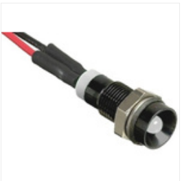
RS PRO Green, Red, Yellow Indicator, 24 V dc, 8mm Mounting Hole Size, Lead Wires Termination, IP67, Индикатор Stock number: 7239523
