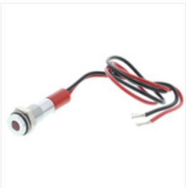
RS PRO Red Indicator, 24 V dc, 6mm Mounting Hole Size, Lead Wires Termination, IP67, Индикатор Stock number: 7001823
