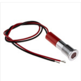
RS PRO Red Indicator, 24 V dc, 8mm Mounting Hole Size, Lead Wires Termination, IP67, Индикатор Stock number: 7001924
