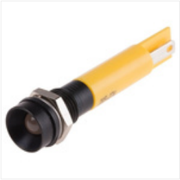
RS PRO Yellow Indicator, 24 V ac/dc, 8mm Mounting Hole Size, Solder Tab Termination, IP67, Индикатор Stock number: 0205274
