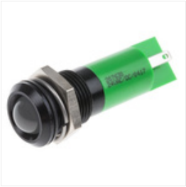
RS PRO Green Indicator, 24 V ac/dc, 14mm Mounting Hole Size, Solder Tab Termination, IP67, Индикатор Stock number: 0207630
