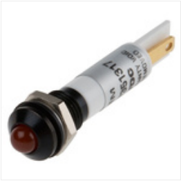
RS PRO Orange Indicator, 21.6 → 26.4 V dc, 8mm Mounting Hole Size, Solder Lug Termination, IP67, Индикатор Stock number: 8432486
