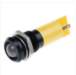
RS PRO Yellow Indicator, 24 V ac/dc, 14mm Mounting Hole Size, Solder Tab Termination, IP67, Индикатор Stock number: 0207501
