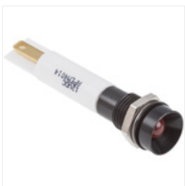
RS PRO Orange Indicator, 10.8 → 13.2 V dc, 8mm Mounting Hole Size, Solder Lug Termination, IP67, Индикатор Stock number: 8432483
