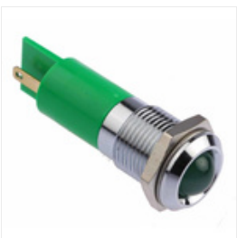
RS PRO Green Indicator, 24 V ac/dc, 14mm Mounting Hole Size, Tab Termination, IP67, Индикатор Stock number: 0207157
