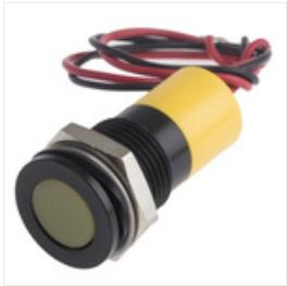
RS PRO Yellow Indicator, 12 V dc, 14mm Mounting Hole Size, Lead Wires Termination, IP67, Индикатор Stock number: 7038986
