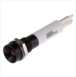
RS PRO Orange Indicator, 21.6 → 26.4 V dc, 8mm Mounting Hole Size, Solder Lug Termination, IP67, Индикатор Stock number: 8432480
