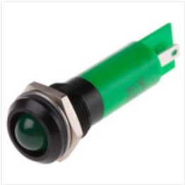
RS PRO Green Indicator, 12 V, 12mm Mounting Hole Size, Solder Tab Termination, IP67, Индикатор Stock number: 0208740
