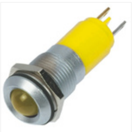
RS PRO Yellow Indicator, 24 V ac/dc, 14mm Mounting Hole Size, Solder Tab Termination, IP67, Индикатор Stock number: 0205476
