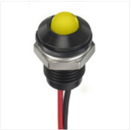
RS PRO Yellow Indicator, 24 V dc, 8mm Mounting Hole Size, Lead Wires Termination, IP67, Индикатор Stock number: 1329140
