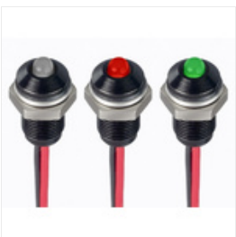
RS PRO Green, Red Panel LED, 10.8 → 13.2 V dc, 6mm Mounting Hole Size, Lead Wires Termination, IP67, Индикатор Stock number: 1713806
