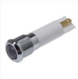
RS PRO White Indicator, 24 V ac/dc, 12mm Mounting Hole Size, Solder Tab Termination, IP67, Индикатор Stock number: 0209052
