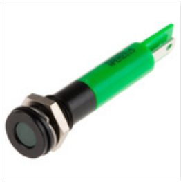
RS PRO Green Indicator, 220 V ac, 8mm Mounting Hole Size, Solder Lug Termination, IP67, Индикатор Stock number: 8462926
