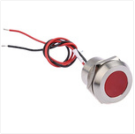
RS PRO Red Indicator, 24 V dc, 22mm Mounting Hole Size, Lead Wires Termination, IP67, Индикатор Stock number: 1232424
