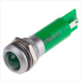
RS PRO Green Indicator, 24 V ac/dc, 12mm Mounting Hole Size, Solder Tab Termination, IP67, Индикатор Stock number: 0205381
