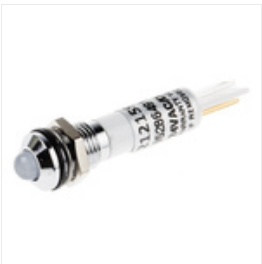
RS PRO White Indicator, 24 V ac/dc, 8mm Mounting Hole Size, Solder Tab Termination, IP67, Индикатор Stock number: 0212159
