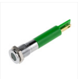
RS PRO Green Indicator, 12 V dc, 8mm Mounting Hole Size, Faston, Solder Lug Termination, IP67, Индикатор Stock number: 8385564
