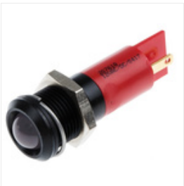
RS PRO Red Indicator, 12 V, 14mm Mounting Hole Size, Solder Tab Termination, IP67, Индикатор Stock number: 0207618
