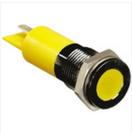
RS PRO Yellow Indicator, 12 V dc, 14mm Mounting Hole Size, Solder Tab Termination, IP67, Индикатор Stock number: 7038875
