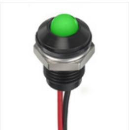
RS PRO Green Indicator, 12 V dc, 8mm Mounting Hole Size, Lead Wires Termination, IP67, Индикатор Stock number: 1329134
