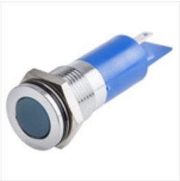
RS PRO Blue Indicator, 6 → 36 V dc, 14mm Mounting Hole Size, Solder Tab Termination, IP67, Индикатор Stock number: 7039046
