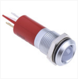
RS PRO Red Indicator, 24 V ac/dc, 14mm Mounting Hole Size, Solder Tab Termination, IP67, Индикатор Stock number: 0206889
