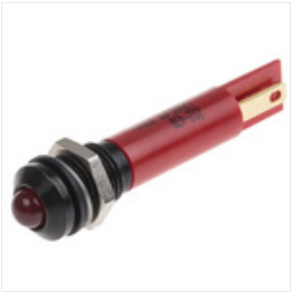
RS PRO Red Indicator, 12 V, 8mm Mounting Hole Size, Solder Tab Termination, IP67, Индикатор Stock number: 0212430
