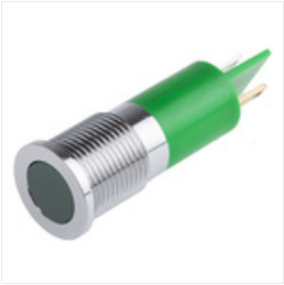
RS PRO Green Indicator, 6 → 36 V dc, 14mm Mounting Hole Size, Solder Tab Termination, IP67, Индикатор Stock number: 7039049
