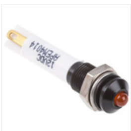
RS PRO Orange Indicator, 21.6 → 26.4 V dc, 6mm Mounting Hole Size, Solder Lug Termination, IP67, Индикатор Stock number: 8432442
