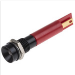
RS PRO Red Indicator, 24 V ac/dc, 8mm Mounting Hole Size, Solder Tab Termination, IP67, Индикатор Stock number: 0212402
