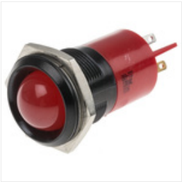
RS PRO Red Indicator, 130 V ac, 22mm Mounting Hole Size, Tab Termination, IP67, Индикатор Stock number: 0209737
