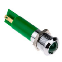
RS PRO Green Indicator, 24 V ac/dc, 12mm Mounting Hole Size, Solder Tab Termination, IP67, Индикатор Stock number: 0208481
