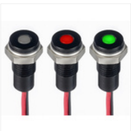
RS PRO Green, Red Panel LED, 1.8 → 3.3 V dc, 6mm Mounting Hole Size, Lead Wires Termination, IP67, Индикатор Stock number: 1713821
