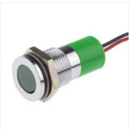
RS PRO Green Indicator, 12 V dc, 14mm Mounting Hole Size, Lead Wires Termination, IP67, Индикатор Stock number: 7038920
