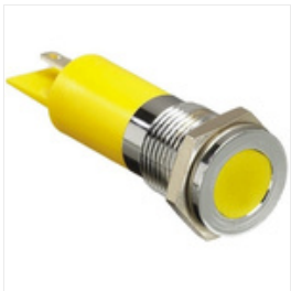
RS PRO Yellow Indicator, 220 V ac, 14mm Mounting Hole Size, Solder Tab Termination, IP67, Индикатор Stock number: 7038850
