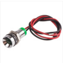
RS PRO Green Indicator, 2 V dc, 8mm Mounting Hole Size, Lead Wires Termination, IP67, Индикатор Stock number: 7239312
