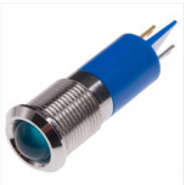
RS PRO Blue neon Indicator, 110 V ac, 14.5mm Mounting Hole Size, Solder Tab Termination, IP40, Индикатор Stock number: 0204366
