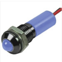
RS PRO Blue Indicator, 2 V dc, 6mm Mounting Hole Size, Lead Wires Termination, IP67, Индикатор Stock number: 7227710
