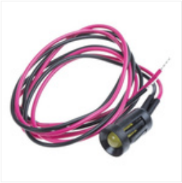
RS PRO Yellow Indicator, 12 V dc, 8mm Mounting Hole Size, Lead Wires Termination, Индикатор Stock number: 0204108
