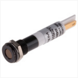
RS PRO Orange Indicator, 10.8 → 13.2 V dc, 8mm Mounting Hole Size, Solder Lug Termination, IP67, Индикатор Stock number: 8432496
