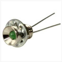
RS PRO Green Indicator, 2 V dc, 6.5mm Mounting Hole Size, Lead Pins Termination, Индикатор Stock number: 1133971
