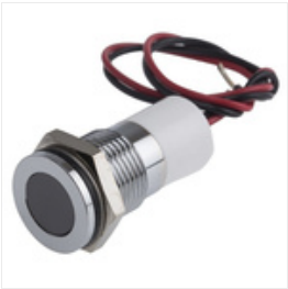
RS PRO White Indicator, 220 V ac, 14mm Mounting Hole Size, Lead Wires Termination, IP67, Индикатор Stock number: 7038973
