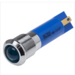
RS PRO Blue Indicator, 230 V ac, 12mm Mounting Hole Size, Tab Termination, IP67, Индикатор Stock number: 0207309
