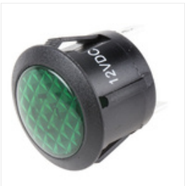
RS PRO Green Incandescent Indicator, 12 V dc, 20.8mm Mounting Hole Size, Faston, Solder Lug Termination, Индикатор Stock number: 7932557
