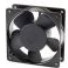
RS PRO, 230 V ac, AC Axial Fan, 120 x 120 x 38mm, 186.9m³/h, 15W
