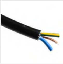
RS PRO 3 Core 1.25 mm 2 Mains Power Cable, Black Polyvinyl Chloride PVC Sheath 100m, 13 A 300 V, 500 V, 3183Y H05VV-F
