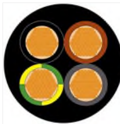
RS PRO 4 Core 4 mm 2 Mains Power Cable, Cross-Linked Compound, Type EM 8 to EN 50363-6 Sheath 100, 750 V, H07ZZ-F
