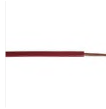
RS PRO Red STRANDED BR Tri-rated Cable, 6 mm 2 CSA, 600 V, 48 A, 100m Stock number: 0359194
