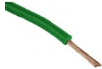
RS PRO Green Tri-rated Cable, 0.75 mm 2 CSA, 1 kV dc, 600 V ac, 14 A, 100m Stock number: 1805968
