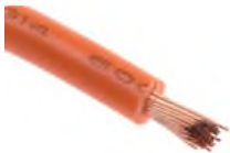
RS PRO Orange Tri-rated Cable, 2.5 mm 2 CSA, 1 kV dc, 600 V ac, 30 A, 100m
