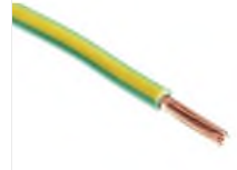
RS PRO Green/Yellow Tri-rated Cable, 4 mm 2 CSA, 1 kV, 41 A, 100m Stock number: 8111445
