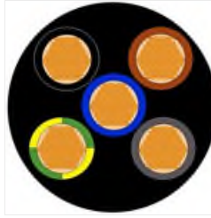
RS PRO 5 Core 1.5 mm 2 Mains Power Cable, Thermoplastic Elastomers TPE Sheath 100m, 22 A 450/750 V, H07RN-F Stock number: 0536219
