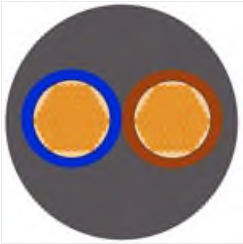
RS PRO 2 Core 0.5 mm 2 Mains Power Cable, Grey Polyvinyl Chloride PVC Sheath 100, 3 A 300 V, 2182Y H03VV-F
