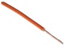
RS PRO Orange Tri-rated Cable, 1 mm 2 CSA, 1 kV dc, 600 V ac, 17 A, 100m
