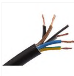
RS PRO 5 Core 0.75 mm 2 Mains Power Cable, Black Polyvinyl Chloride PVC Sheath 100m, 6 A 300 V, 500 V, 3185Y H05VV-F
