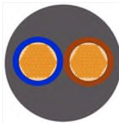
RS PRO 2 Core 0.75 mm 2 Mains Power Cable, Grey Polyvinyl Chloride PVC Sheath 100, 6 A 300 V, 500 V, 3182Y H05VV-F
