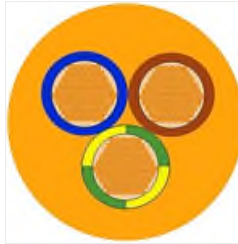
RS PRO 3 Core 1.25 mm 2 Mains Power Cable, Orange Polyvinyl Chloride PVC Sheath 100m, 13 A 500 V, 3183Y H05VV-F
