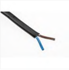
RS PRO 2 Core 0.5 mm 2 Mains Power Cable, Black Polyvinyl Chloride PVC Sheath 100m, 3 A 300 V, 2192Y H03VVH2-F
