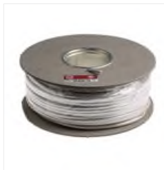
RS PRO 2 Core 0.5 mm 2 Mains Power Cable, White Polyvinyl Chloride PVC Sheath 100m, 3 A 300 V, 2192Y H03VVH2-F
