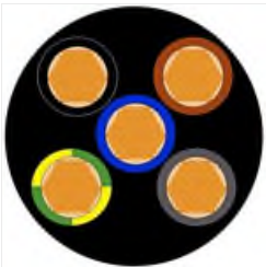
RS PRO 5 Core 1.5 mm 2 Mains Power Cable, Black Polyvinyl Chloride PVC Sheath 100m, 16 A 500 V, 3185Y H05VV-F Stock number: 0491982
