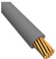
RS PRO Grey Tri-rated Cable, 1 mm 2 CSA, 1 kV dc, 600 V ac, 17 A, 100m
