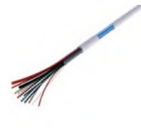
RS PRO 8 Core Screened Security Cable 2 x 0.75 mm 2 , 6 x 0.22 mm 2 CSA, Polyvinyl Chloride PVC Sheath, 100m, Кабель Stock number: 1368145
