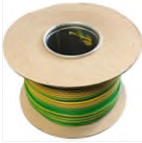
RS PRO Single Core Cable HO7Z-R Conduit & Trunking Cable, 25 mm 2 CSA , 450 V dc, 750 V ac, Green/Yellow LSZH 100m, Кабель
