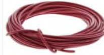
RS PRO Unshielded Test Lead Wire 0.5 mm 2 CSA 500 V, Red PVC, 100 Strands ,Length 5m, Провод Stock number: 7482002
