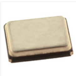
RS PRO 10MHz Crystal \pm 50\text{ppm} SMT 4-Pin 3.2 x 2.5 x 0.7mm
