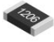
RS PRO 33Ω, 1206 (3216M) Thick Film SMD Resistor ±5% 0.25W Код товара RS 713-1265
