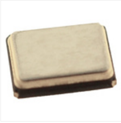
RS PRO 25MHz Crystal \pm 30 ppm SMT 4-Pin 3.2 x 2.5 x 0.7mm
