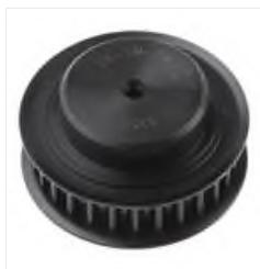
RS PRO Timing Belt Pulley, Steel 9mm Belt Width x 5mm Pitch, 28 Tooth, Зубчатый шкив
