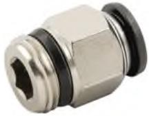
RS PRO Threaded-to-Tube Pneumatic Fitting, R 1/2 to, Push In 8 mm, 20 bar, Прямой фитинг
