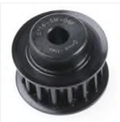
RS PRO Timing Belt Pulley, Steel 9mm Belt Width x 5mm Pitch, 16 Tooth, Зубчатый шкив
