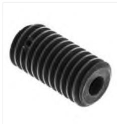
RS PRO Steel RH 30mm Long Worm Gear, 1 Start , 15.6mm Diam , 14mm Pitch Diam. , 20° Pressure Angle
