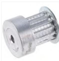
RS PRO Timing Belt Pulley, Aluminium 6mm Belt Width x 2.5mm Pitch, 14 Tooth, Зубчатый ШКИВ
