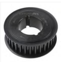
RS PRO Timing Belt Pulley, Steel 28mm Belt Width x 8mm Pitch, 30 Tooth, Зубчатый шкив
