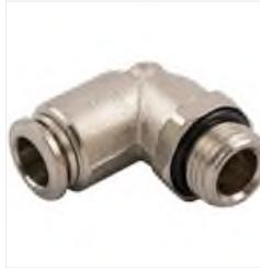
RS PRO Threaded-to-Tube Pneumatic Elbow Fitting G 1/4 to Push In 8 mm, 20bar
