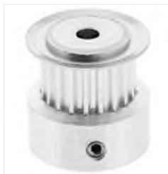
RS PRO Timing Belt Pulley, Aluminium, Zinc Plated Steel 6.35mm Belt Width x 2.032mm Pitch, 20 Tooth, Зубчатый шкив
