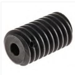
RS PRO Bronze, Steel RH 32mm Long Worm Gear, 2 Start , 18mm Diam , 16mm Pitch Diam. , 20° Pressure Angle
