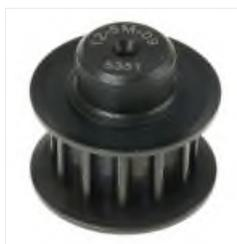
RS PRO Timing Belt Pulley, Steel 9mm Belt Width x 5mm Pitch, 12 Tooth, Зубчатый шкив
