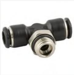
RS PRO Threaded-to-Tube Tee Connector Push In 8 mm x Push In 8 mm x G 1/4 20 bar, ФИТИНГ
