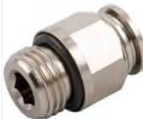
RS PRO Threaded-to-Tube Pneumatic Fitting, G 1/4 to, Push In 6 mm, 20bar
