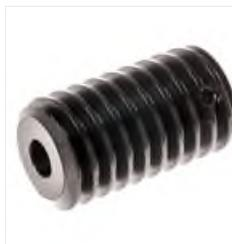
RS PRO Steel RH 32mm Long Worm Gear, 1 Start , 18mm Diam , 16mm Pitch Diam. , 20° Pressure Angle
