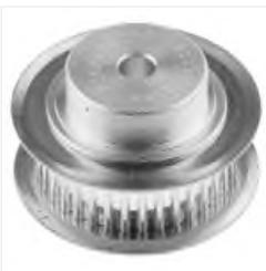
RS PRO Timing Belt Pulley, Aluminium, Zinc Plated Steel 6.35mm Belt Width x 2.032mm Pitch, 36 Tooth, Зубчатый шкив
