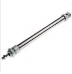
RS PRO Pneumatic Roundline Cylinder 20mm Bore, 200mm Stroke, ISO 6432 Series, Double Acting, Пневмоцилиндр
