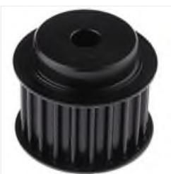
RS PRO Timing Belt Pulley, Steel 30mm Belt Width x 8mm Pitch, 22 Tooth, Зубчатый шкив
