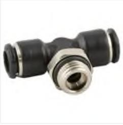
RS PRO Threaded-to-Tube Tee Connector Push In 10 mm x Push In 10 mm x G 1/4 20 bar, ФИТИНГ
