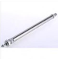
RS PRO Pneumatic Roundline Cylinder 16mm Bore, 200mm Stroke, ISO 6432 Series, Double Acting, Пневмоцилиндр
