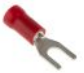
RS PRO Insulated Crimp Spade Connector, 0.5mm 2 to 1.5mm 2 , 22AWG to 16AWG, M3.5 Stud Size Vinyl, Red Код товара RS 534-272
