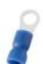
RS PRO Insulated Ring Terminal, 4.3mm Stud Size, 1.5mm 2 to 2.5mm 2 Wire Size, Blue Код товара RS 178-8679
